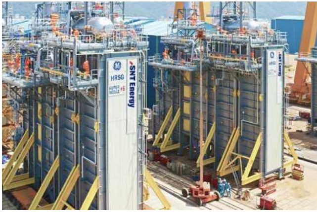
Heat Recovery Steam Generator
