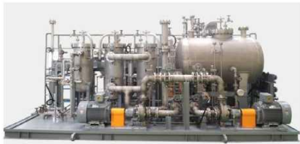
Seal Oil Unit
