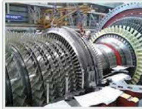
Blade Ring Assembly & Clearance Check
