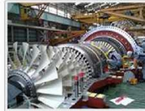
Blade Ring Assembly & Bolt Tightening
